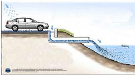
The Morton Arboretum's environmentally friendly parking lot contrasts sharply with traditional parking lots where rain washes dirt and oil from cars off the asphalt and into storm drains. Since there is no filtering system in the traditional parking lot, the water from the storm drains empties into nearby streams, where it is carried into local lakes and groundwater. The
