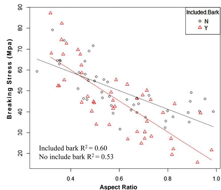
**Figure 5.** Breaking stress plotted against aspect ratio
