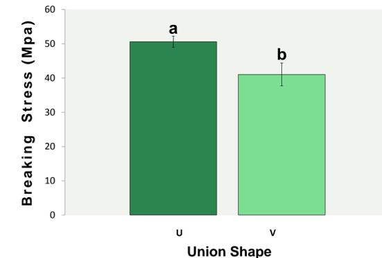
**Figure 7.** Average breaking stress between union shapes
