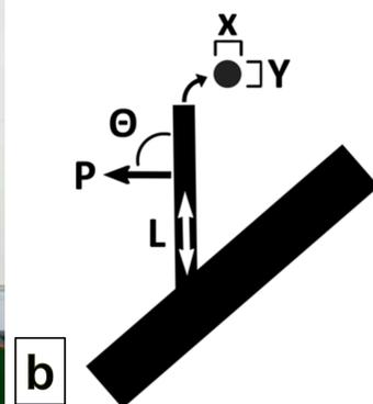
**Figure 4.** a) The branch breaking apparatus set up with a branch union. b) A free body diagram illustrating the variables represented in the stress equation: P is the maximum load (kN), L is the distance from branch attachment to pull point(m),  $\Theta$  is the angle between the branch and cable, and x and y are in-line and perpendicular diameters (m) respectively.
