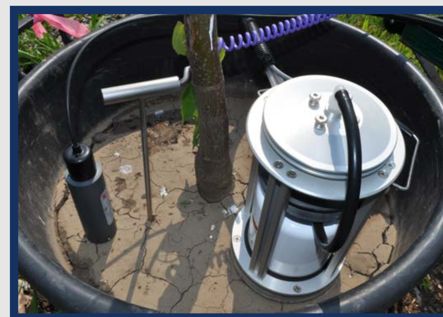
Image 2. Soil moisture probe, temperature probe, and LI-8100A
