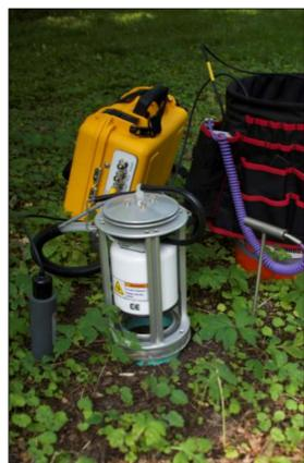
**Figure 3.** Surface respiration with Licor 8100A.
